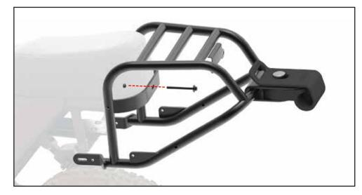
1 Remove PEDAL battery. Align central mounting hole of Quickrack with the rear of your PEDAL seat. Thread M5 x 45mm bolt through Quickrack through bike frame and secure locknut.
