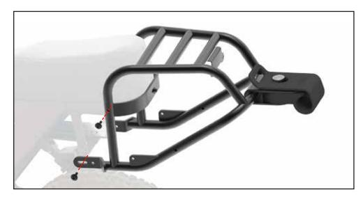
2 Insert 2pcs M5 x 20mm bolts through the Quickrack and into side mounting holes on bike frame. Repeat x's 2 on opposite side of the Quickrack. Don't overtighten.
