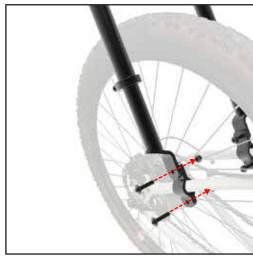
4 Thread bolts through the extender tube. through the clamp brackets and into the locknuts, tighten firmly. Repeat on the other side.
