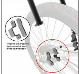
fork frame. Position the clamp brackets over the gasket and frame.
