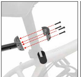
2 Place rubber gasket around bike seat tube. 3 Place rubber gasket over your bikes rear Thread 4 bolts through the loose side of the C-clamp and tighten to the rack side of the C-clamp.
