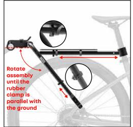
1 Loosen set screws, adjust the seat tube extender and rear fork extender so that they align with your bikes frame. Make sure the Quickrack rubber clamp is parallel with the ground. Tighten set screws.
